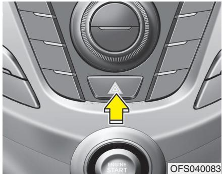
It should be used whenever emergency repairs are being made or when the vehicle is stopped near the edge of a roadway.
